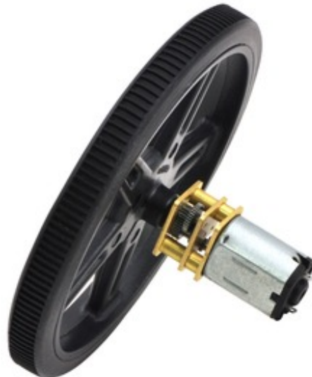
Black Pololu 70x8mm wheel on a Pololu micro metal gearmotor.
