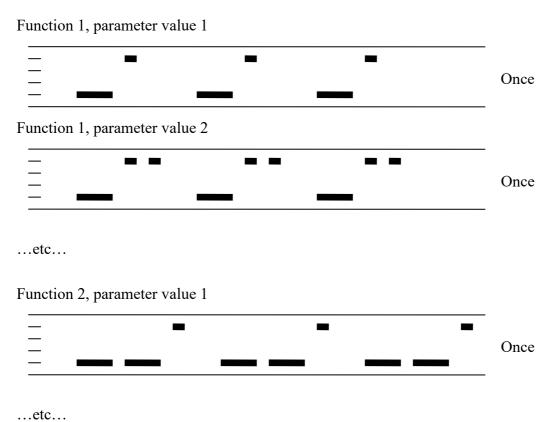
If the throttle stick is moved to zero during one of the above sequences, the parameter value of that function is selected and stored. And you will hear this sound:
