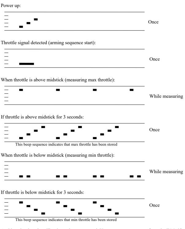
At this point throttle calibration values are stored. You may remove power from the ESC, if you just wanted to do a throttle calibration and not enter programming mode.
