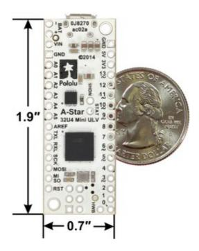
This version, the A-Star Mini ULV, can be powered from a 0.5 V to 5.5 V external source. The input voltage is regulated to 5 V by a TPS61202 switching step-up (boost) converter from Texas Instruments. (We also make a standalone regulator based on this integrated circuit.)
