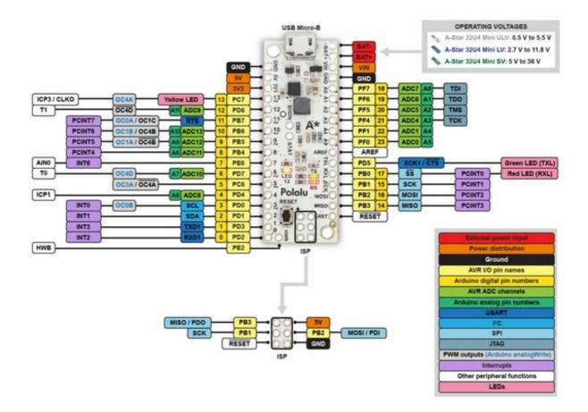
This diagram identifies the I/O and power pins on the A-Star 32U4 Mini (even though it shows the ULV version, it applies to all three A-Star Mini boards); it is also available as a printable PDF (269k pdf). For more information about the ATmega32U4 microcontroller and its peripherals, see Atmel's ATmega32U4 documentation.
