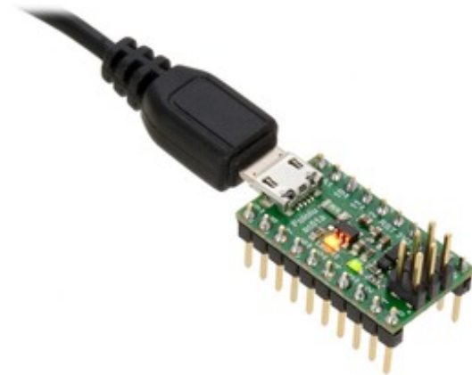
A-Star 32U4 Micro with soldered headers and connected USB cable.
