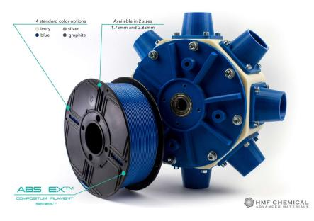
ABS materials are dedicated for industry and professional application in close chamber FDM 3D printers. ABS EX™ filaments are marked by excellent cohesion of layers and very low linear contraction (up to 0,4%). Thanks to it the difference in mechanical properties of the printed sample compared to the model produced by the injection method is only 8%. Additionally, ABS EX™ characterized by excellent machining processing: turning, milling, threading etc.
