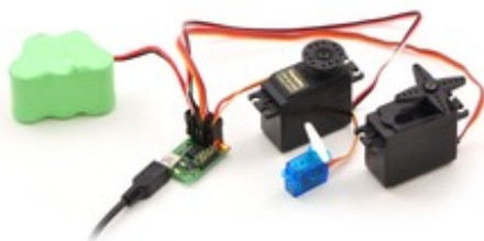
Micro Maestro 6-channel USB servo controller (fully assembled) controlling three servos.
