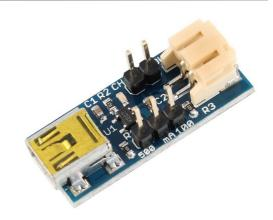
This small circuit can recharge in an extremely simple way Li-Po and Li-Ion cells. Using a jumper with two positions you can select two possible values for the charging current, 100mA and 500mA; the correct value should be chosen in consultation with the characteristics of the battery.
