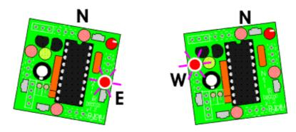
Interfacing to the beacon is simple — it has four digital outputs that indicate which of its four sides detects the other beacon the strongest. You can establish the direction to another beacon to within a few degrees by rotating the beacon back and forth and noting the point where the output switches from one side to another. An enable input lets you select between active mode and a low-power mode.
