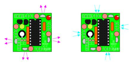
The transmit and detect cycle is carried out more than one thousand times per second, and a small microcontroller monitors all four detectors to decide the direction to the other beacon. The beacons have four red LEDs that indicate the direction to the other beacon; if you take two beacons and rotate them, the LEDs will always keep lighting up in the direction of the other beacon.
