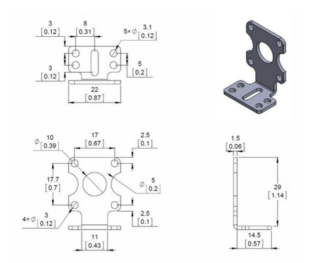
Mechanical drawing for the Pololu extended stamped aluminum L-bracket for plastic gearmotors. Units are mm over [inches].
