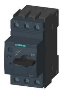
CIRCUIT-BREAKER SZ S0, FOR MOTOR PROTECTION, CLASS 10, A-RELEASE 20...25A, N-RELEASE 325A, SCREW CONNECTION, STANDARD SW. CAPACITY,
