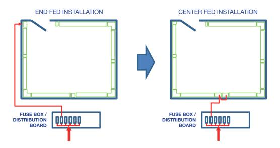
Always consider the size and position of the likely electrical loads. This will dictate the number of wiring circuits and the length and position of each power track.
