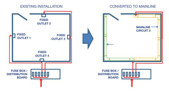
Making use of Mainline's 32Amp capability may be possible in some applications. In these cases the wiring and circuit protection must be upgraded to comply with wiring and installation requirements.
