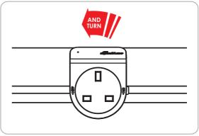
**Important:** To reposition adaptors / sockets the user must rotate and completely remove the adaptor / socket from the track before inserting in the new position. Sockets/adaptors must not be pushed, dragged or forced along the track in any way.
