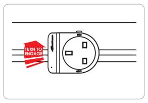
To remove a socket, turn 90° anti- clockwise until the socket releases from the track.
