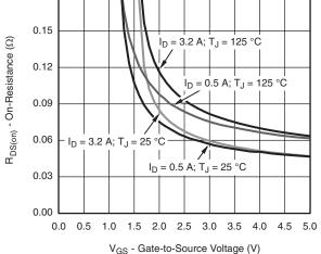
On-Resistance vs. Gate-to-Source Voltage
