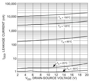
Fig. 9 Typical Leakage Current vs. Drain-Source Voltage
