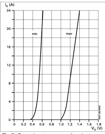
**Fig. 7** Forwarde gate current vs. forard gate voltage.
