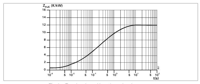
**Fig. 1** Transient thermal impedance, junction to case.
