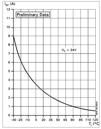
Fig. 8 Gate trigger current vs. junction temperature
