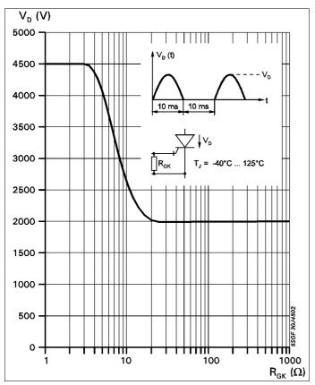
**Fig. 5** Forward blocking voltage vs. gate-cathode resistance.
