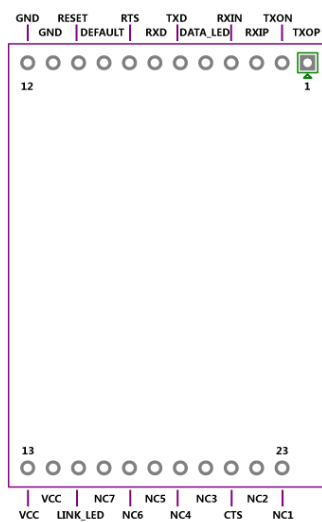
Figure 2-2 W7500S2E-R1 pinout
