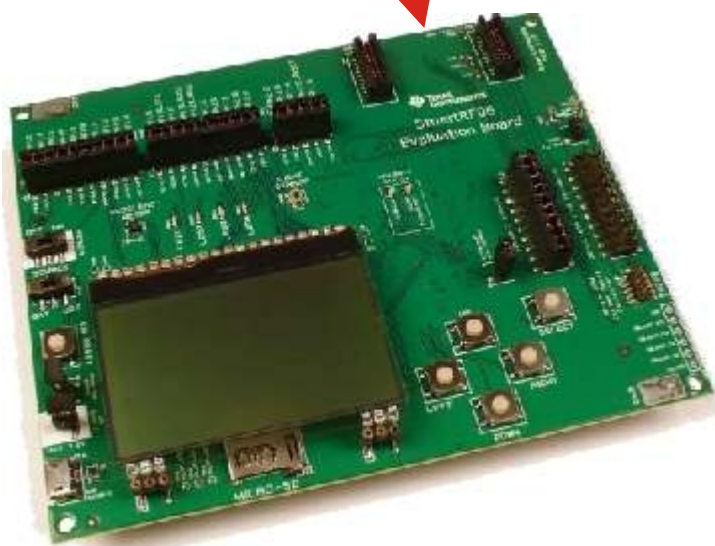
SMART RF06 Evaluation board (TI)
