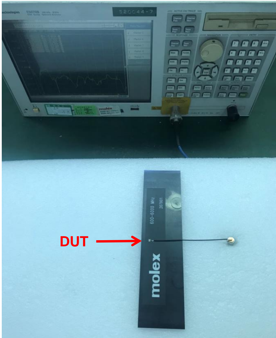
FIGURE4.1.2 ANTENNA LOADED WITH PC/ABS BLOCK OF 1.5MM THICKNESS TESTED WITH VNA E5071C
