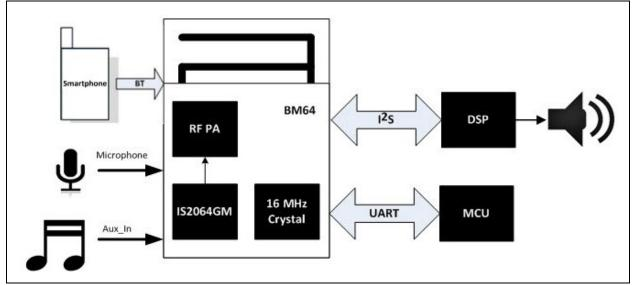
Figure 1-3 illustrates the Multi-speaker application using the BM64 module.
