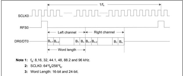
Figure 8-3 illustrates the timing diagram of the audio interface.
