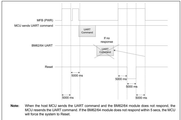
FIGURE 5-7: TIMING SEQUENCE OF POWER DROP PROTECTION
