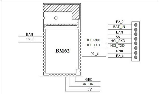
Configuration and firmware programming modes are entered according to the system configuration I/O pins. Table 5-1 provides the system configuration settings. The P2\_0, P2\_4 and EAN pins have internal pull up.
