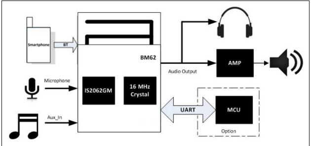
Figure 1-2 illustrates a typical example of the Class 1 BM64 module, which is connected to an external MCU and a DSP/codec.
