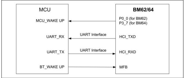
An external MCU can control the BM62/64 module over the UART interface and wakeup the module with the MFB, P0\_0 (BM62) and P3\_7 (BM64) pins.
