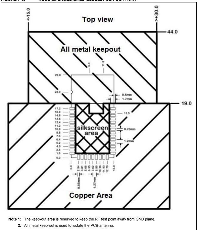
Figure 7-4 illustrates the recommended PCB footprint of the BM64 module.
