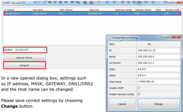
If **Remote Config** is disabled (enabled by default), it is necessary to configure the device by changing the computer's subnet (chapter 6.2).
