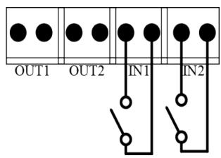
Illustration of the inputs arrangement
