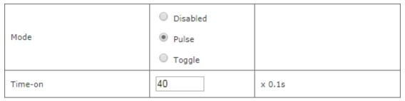
Often this mode is used to maintain power supply for a machinery which is active only when an authorized employee logs in using a card reader. Likewise, it is used in hotel systems. Hotel rooms are often powered after a card is seen by a reader \*special purpose housing.
