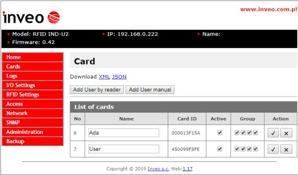
To add a new user card, on the **Cards** tab, click the **Add User by reader** button, and then approximate the card to the reader. The assignment of the card will be signalized by the appropriate beep.
