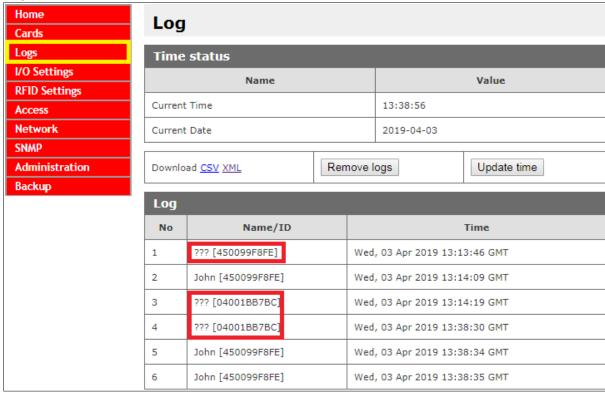
Marked in the log table, cards ID data is an example of unrecognized cards which are not registered in the reader's memory or the card is inactive.
