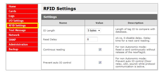
**ID Length** – length of ID code for comparison with cards database **Read Delay** – value of read delay for a consecutive tag multiplied by 0.1s (150 = 15 seconds)
