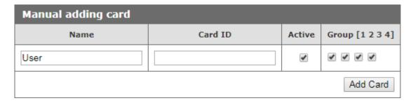
In the window above, just give the user name, enter the ID of the card and assign to the appropriate groups. The entered data confirm the **Add Card** button.
