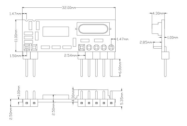
Figure 2: RFM83 DIP mechanical dimension
