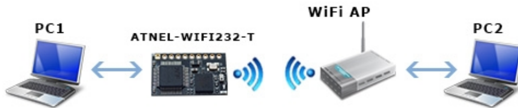
Figure 20. STA Interface Debug Connection
