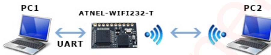
Figure 21. AP Interface Debug Connection
