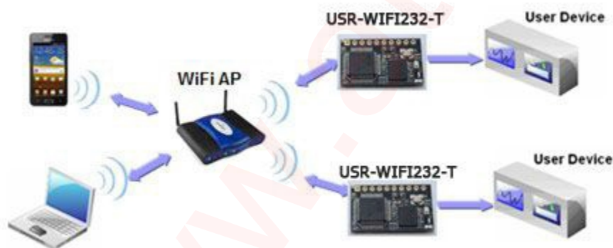
Figure 6. ATNEL-WIFI232-T Basic Wireless Network Structure.
