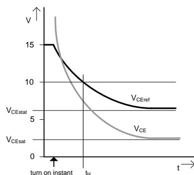
After  $t_{bl}$  has passed, the  $V_{CE}$  monitoring will be triggered as soon as  $V_{CE} > V_{CEref}$  and will turn off the IGBT. The error memory will be set, and the output PRIM\_HOLD\_OUT changes to the HIGH state. Possible failure modes are shown in the following pictures.
