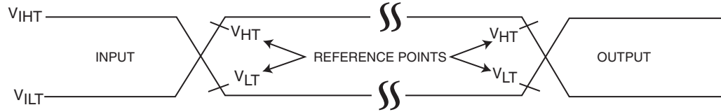
FIGURE 8-5: AC INPUT/OUTPUT REFERENCE WAVEFORMS
