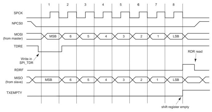
Figure 27-9 shows the behavior of Transmission Register Empty (TXEMPTY), End of RX buffer (ENDRX), End of TX buffer (ENDTX), RX Buffer Full (RXBUFF) and TX Buffer Empty (TXBUFE) status flags within the SPI\_SR during an 8-bit data transfer in Fixed mode with the PDC involved. The PDC is programmed to transfer and receive three units of data. The next pointer and counter are not used. The RDRF and TDRE are not shown because these flags are managed by the PDC when using the PDC.
