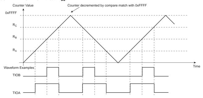
Figure 34-13. WAVSEL = 01 with Trigger
