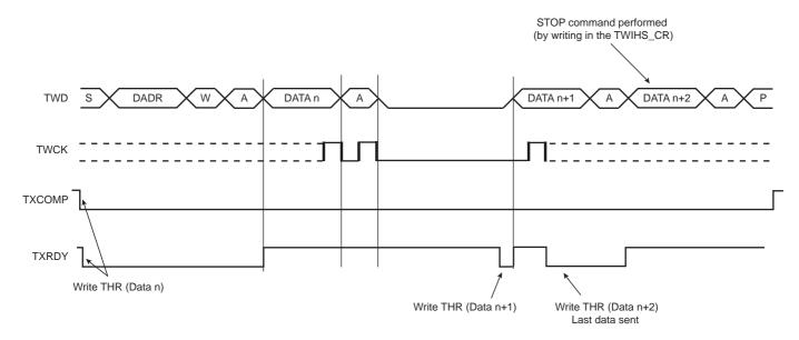
Figure 28-9. Master Write with One Byte Internal Address and Multiple Data Bytes
