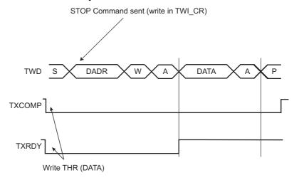
Figure 29-6. Master Write with Multiple Data Bytes
