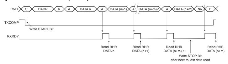
Figure 29-10. Master Read Wait State with Multiple Data Bytes
