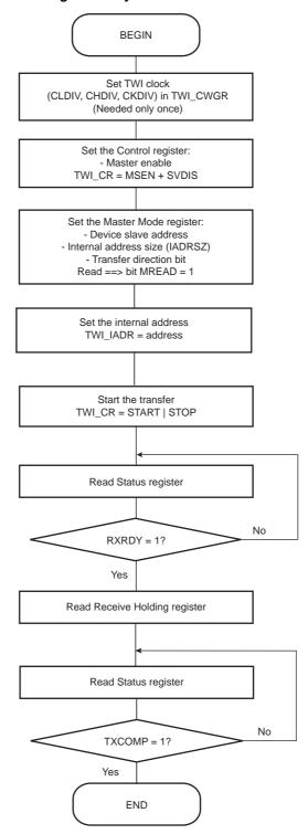
Figure 29-20. TWI Read Operation with Multiple Data Bytes with or without Internal Address
