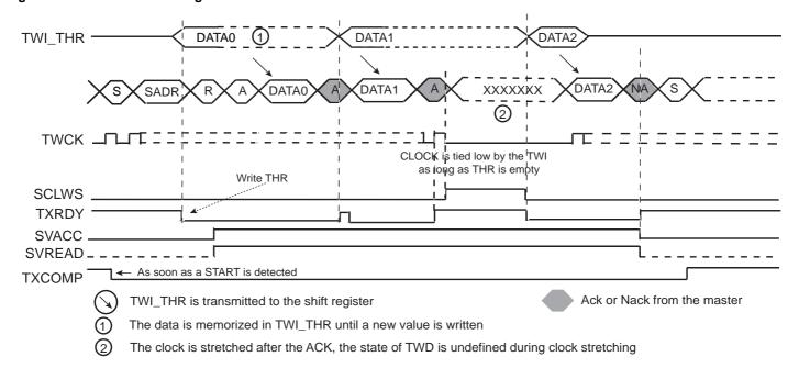
Notes: 1. TXRDY is reset when data has been written in the TWI\_THR to the internal shifter and set when this data has been acknowledged or non acknowledged.
