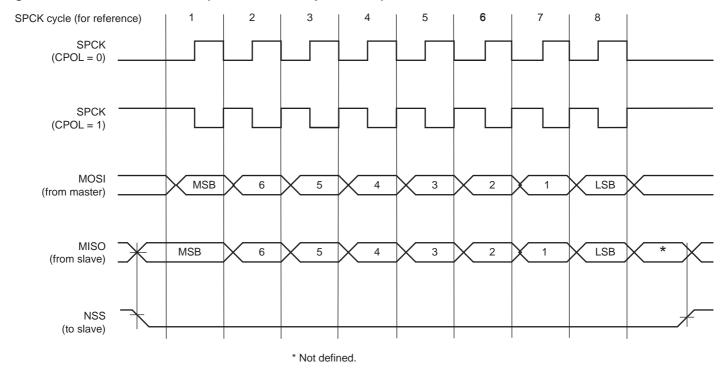
Figure 27-4. SPI Transfer Format (NCPHA = 0, 8 bits per transfer)
