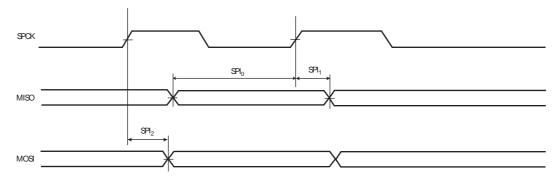
Figure 36-12. SPI Master Mode with (CPOL = 0 and NCPHA=1) or (CPOL=1 and NCPHA= 0)
