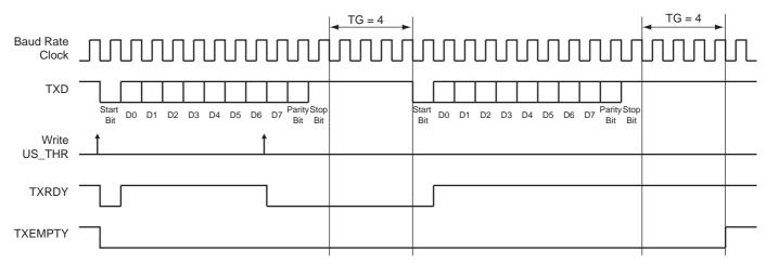
Table 33-6 indicates the maximum length of a timeguard period that the transmitter can handle in relation to the function of the baud rate.
