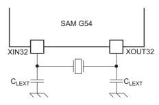
$C_{LEXT} = 2 \times (C_{CRYSTAL} - C_{PARA} - C_{PCB}).$
