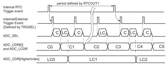
Notes: ADC\_SEL: Command to the ADC analog cell
