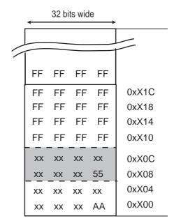
Step 1: Flash array after programming first byte (0xAA) 64-bit used at address 0xX00 (write latch buffer + WP)
