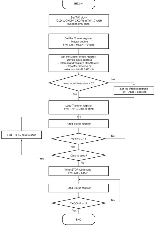
Figure 29-18. TWI Read Operation with Single Data Byte without Internal Address
