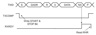
Figure 29-9. Master Read with Multiple Data Bytes
