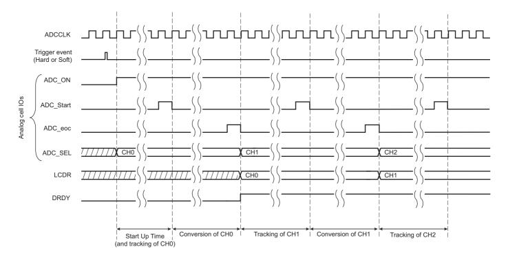
Figure 35-2. Sequence of ADC Conversions
