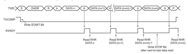
Figure 28-12. Master Read Clock Stretching with Multiple Data Bytes
