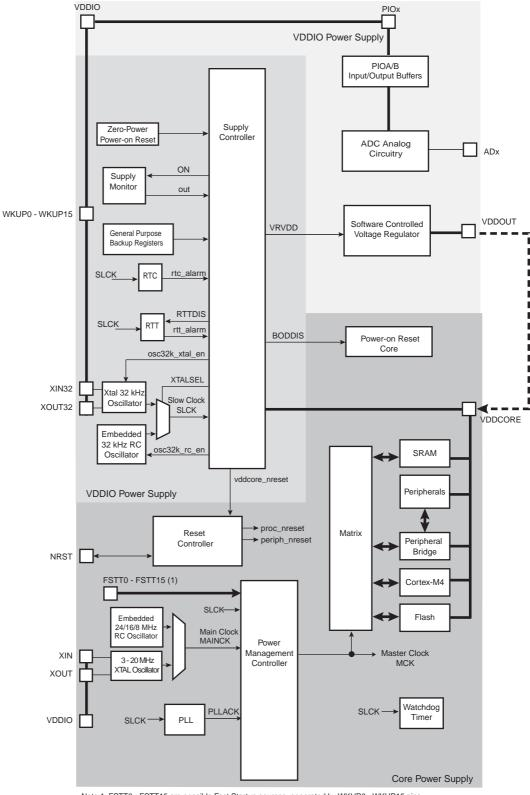
Note 1: FSTT0 - FSTT15 are possible Fast Startup sources, generated by WKUP0 - WKUP15 pins, but are not physical pins.
