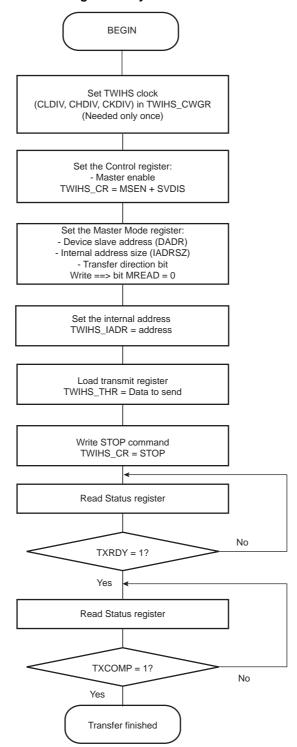
Figure 28-19. TWIHS Write Operation with Multiple Data Bytes with or without Internal Address
