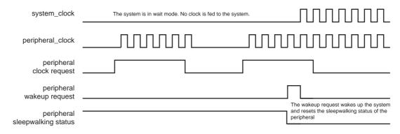
When the system is in Active mode, peripherals enabled for asynchronous partial wake-up have their respective clocks stopped until the peripherals request a clock. When a peripheral requests the clock, the PMC provides the clock without CPU intervention.
