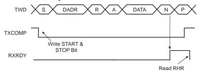
Figure 28-11. Master Read with Multiple Data Bytes
