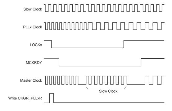
Figure 24-10. Programmable Clock Output Programming
