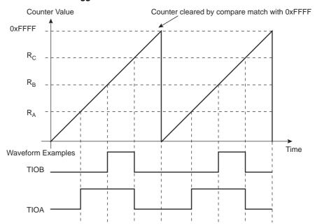
Figure 34-9. WAVSEL= 00 with Trigger
