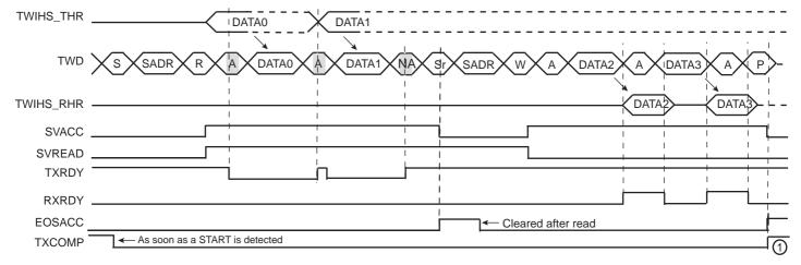
Note: 1. TXCOMP is only set at the end of the transmission. This is because after the REPEATED START, SADR is detected again.
