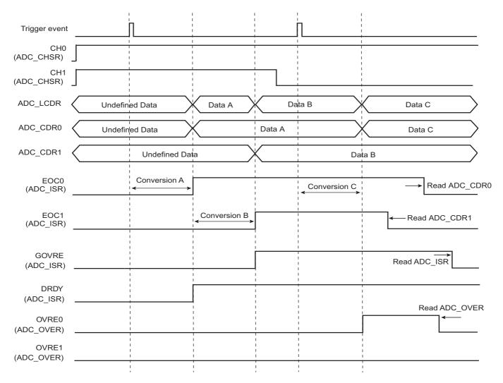
**Warning:** If the corresponding channel is disabled during a conversion or if it is disabled and then reenabled during a conversion, its associated data and corresponding EOCx and GOVRE flags in ADC\_ISR and OVREx flags in ADC\_OVER are unpredictable.
