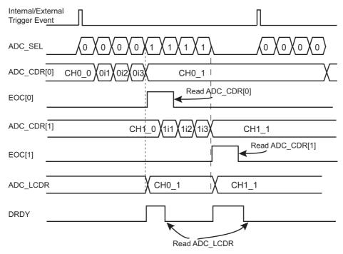
Note: ADC\_SEL: Command to the ADC analog cell
