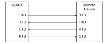
Setting the USART to operate with hardware handshaking is performed by writing the USART\_MODE field in US\_MR to the value 0x2.
