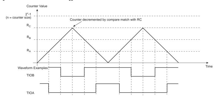
Figure 34-15. WAVSEL = 11 with Trigger
