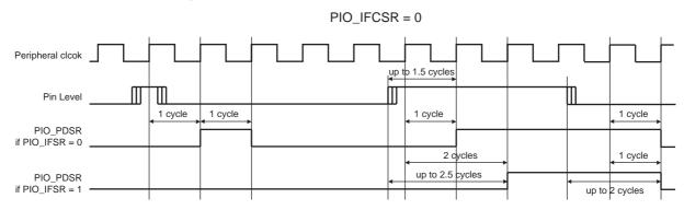
Figure 26-5. Input Debouncing Filter Timing
