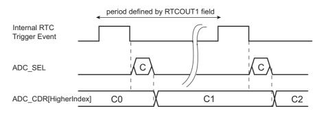
Note: ADC\_SEL: Command to the ADC analog cell
