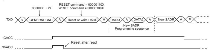
Note: This method allows the user to create a personal programming sequence by choosing the programming bytes and the number of them. The programming sequence has to be provided to the master.
