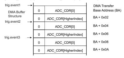
If the last channel is driven by a device with a slower variation compared to other channels (temperature sensor for example), the channel can be enabled/disabled at any time. However, this may not be optimal for downstream processing.
