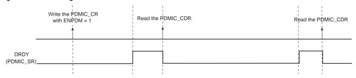
If PDMIC\_CDR is not read before further incoming data is converted, the Overrun Error (OVRE) flag is set in PDMIC\_ISR. Likewise, new data converted when DRDY is high sets the OVRE bit (Overrun Error) in PDMIC\_ISR. In case of overrun, the newly converted data is lost.
