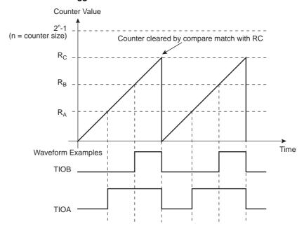
Figure 34-11. WAVSEL = 10 with Trigger
