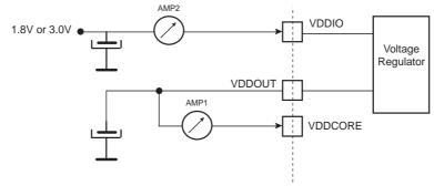
Table 36-11 and Table 36-12 provide Active mode current consumption under typical conditions running the Fibonacci algorithm.
