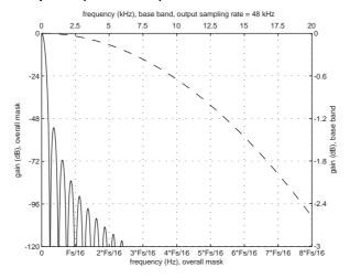
The zeros of this filter are located at multiples of Fs/64.
