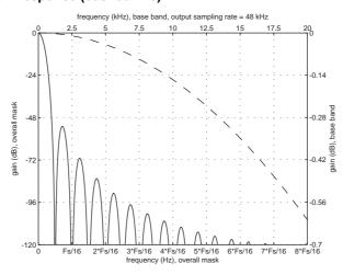
The zeros of this filter are located at multiples of Fs/32
