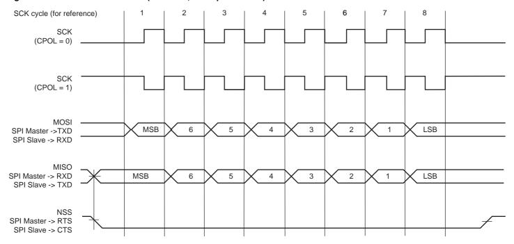
Figure 33-24. SPI Transfer Format (CPHA = 0, 8 bits per transfer)
