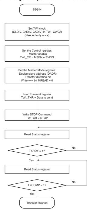
Figure 29-16. TWI Write Operation with Single Data Byte and Internal Address
