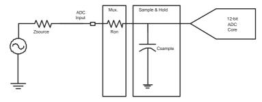
During the tracking phase, the ADC must track the input signal during the tracking time shown below:
