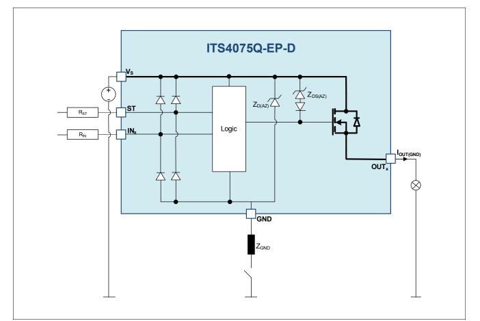
$Z_{GND}$  is recommended to be a resistor in series to a diode.
