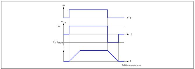
Figure 9 Switching an Inductive Load Timing
