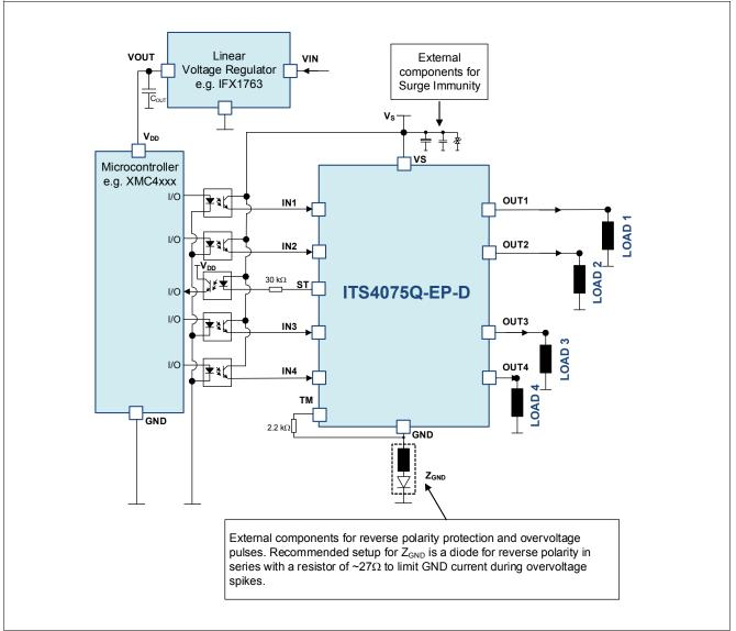
Figure 21 Application Diagram with ITS4075Q-EP-D
