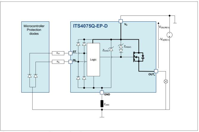
Figure 17 Reverse Polarity Protection with External Components
