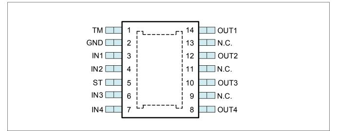
Figure 2 Pin Configuration PG-TSDSO-14
