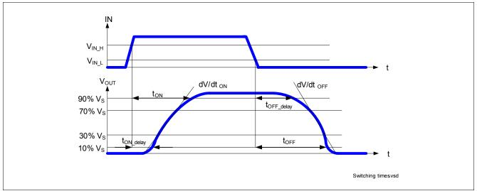
Figure 7 Switching a Resistive Load Timing
