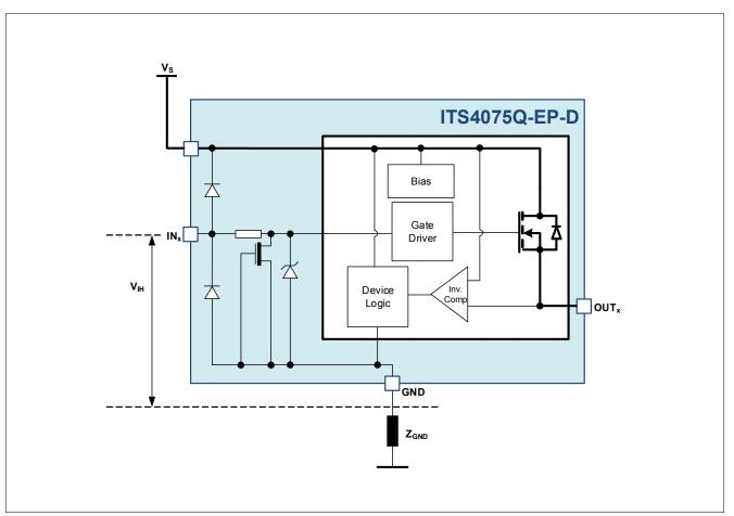
Figure 20 Input Pin Circuitry
