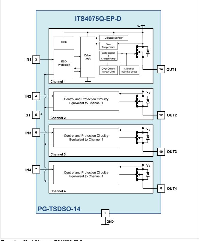
Figure 1 Block Diagram: ITS4075Q-EP-D
