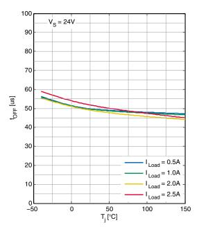
Turn-OFF delay time  $t_{OFF\_delay}$  to  $V_{OUT} = 10\%$  versus Junction Temperature  $T_i$
