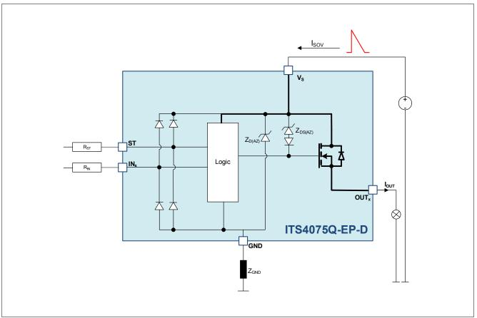
Figure 16 Overvoltage Protection with External Components
