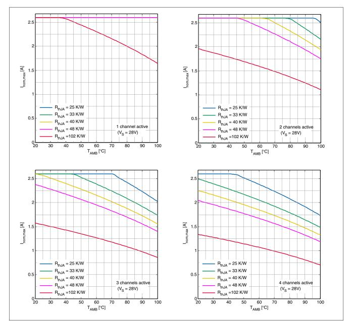
Figure 22 Possible thermal derating of nominal current due to insufficient cooling capability of PCB
