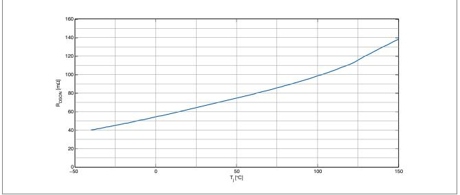
Figure 6 Typical ON-state Resistance
