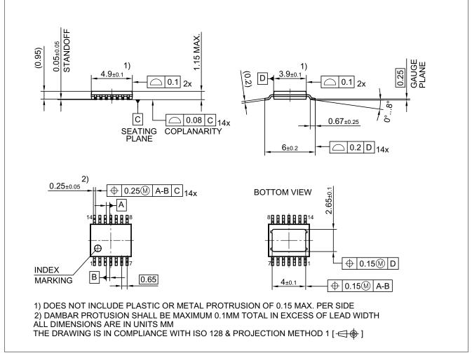
Figure 23 PG-TSDSO-14 (Plastic Dual Small Outline Package) (RoHS-Compliant)
