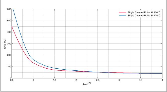
Figure 10 Maximum Energy Dissipation Single Pulse for a Single Channel;  $V_{\rm S}$  = 28 V
