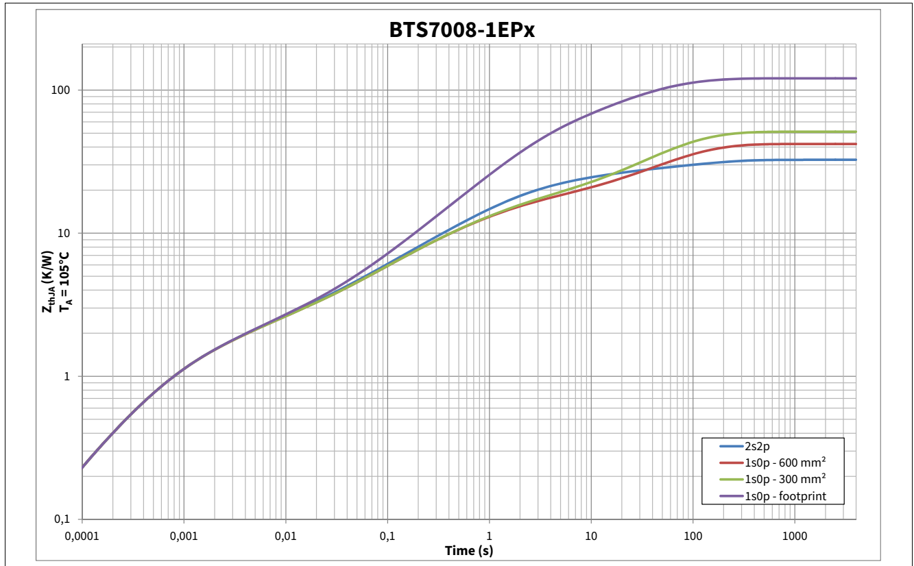
Figure 9 Typical Thermal Impedance. PCB setup according Chapter 4.4.1
