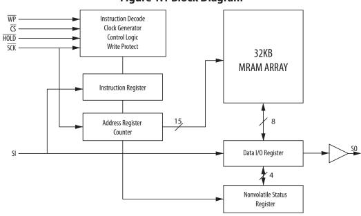
**Figure 1.1 Block Diagram**
