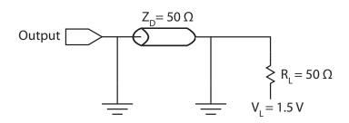
Figure 4.2 Output Load for all Other Parameter Measurements
