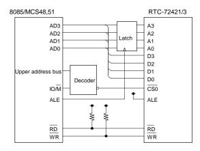
The resistors on the RD and WR lines are not necessary if the CPU does not have a HALT or HOLD state.
