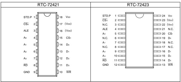
The (VDD) pins are at the same electrical level as VDD. Do not connect these pins externally. The N.C. pins are not connected internally. Ground them in order to prevent noise.
