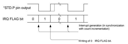
The output levels of the STD.P pin are low (down) and open circuit (up).
