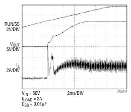
Figure 17. LTC3703 Startup Operation
