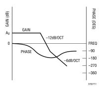
Figure 11. Transfer Function of Buck Modulator
