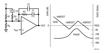
Figure 14. Type 3 Schematic and Transfer Function
