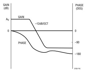
Figure 16. Transfer Function of Boost Modulator
