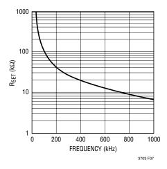
Figure 7. Timing Resistor (R<sub>SET</sub>) Value
