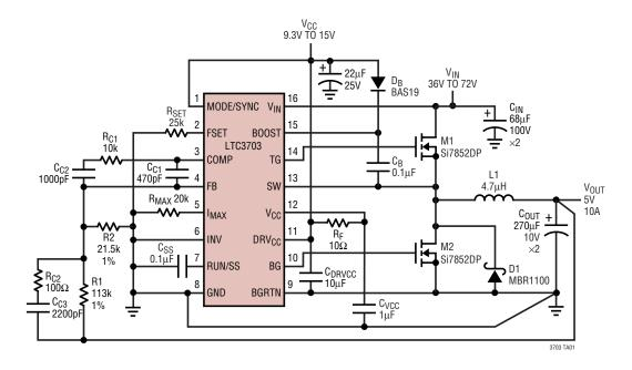
Single Input Supply 12V/5A Output Step-Down Converter
