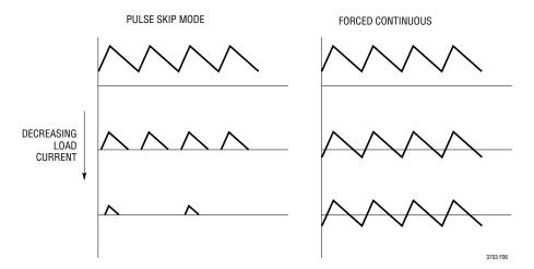
Figure 6. Comparison of Inductor Current Waveforms for Pulse Skip Mode and Forced Continuous Operation
