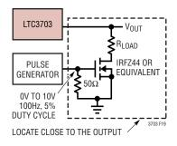
Figure 19. Transient Load Generator
