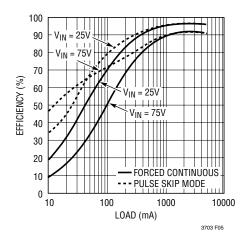
Figure 5. Efficiency in Pulse Skip/Forced Continuous Modes
