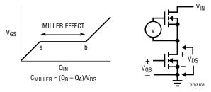
Figure 9. Gate Charge Characteristic
