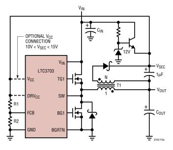
Figure 10c. Secondary Output Loop and  $V_{CC}$  Connection
