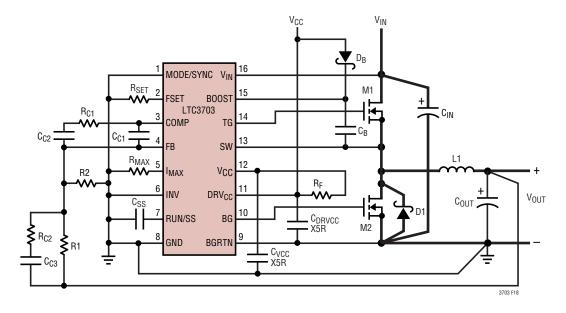
Figure 20. LTC3703 Buck Converter Suggested Layout
