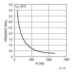
Figure 2. Frequency vs R<sub>T</sub>
