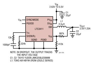
Figure 1. Step-Down 2.5V/1.25A Regulator
