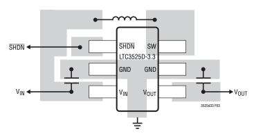
Figure 3. Recommended Component Placement
