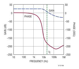
Figure 9. Converter Bode Plot,  $V_{IN} = 3.5V$ ,  $I_{LOAD} = 1A$
