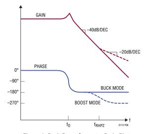
Figure 4. Buck-Boost Converter Bode Plot
