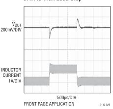
$5V_{IN}$  to  $5.0V_{OUT}$ Burst to PWM Waveforms,
