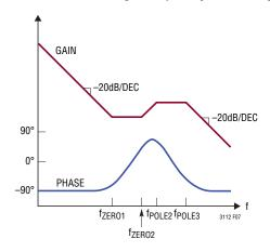
Figure 7. Type III Compensation Bode Plot.
