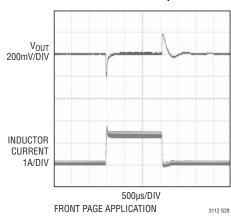
12V<sub>IN</sub> to 5V<sub>OUT</sub> 0.1A to 1.0A Load Step
