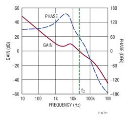
Figure 11. Complete Loop Bode Plot.
