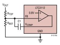
Figure 5. Error Amplifier with Type I Compensation
