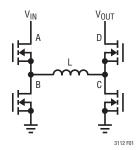
Figure 1. Buck-Boost Switch Topology
