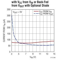
**Burst Mode No-Load Input Current**
