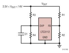
Figure 2. Setting the Output Voltage
