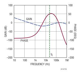
Figure 10. Compensated Error Amplifier Bode Plot.
