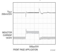
5V<sub>IN</sub> to 5V<sub>OUT</sub> 0.1A to 1.0A Load Step
