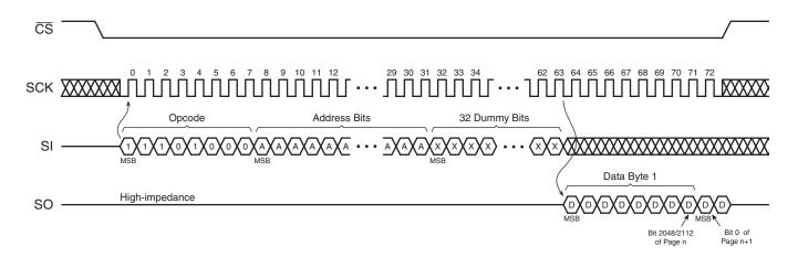
Figure 25-2. Continuous Array Read (Opcode 0Bh)
