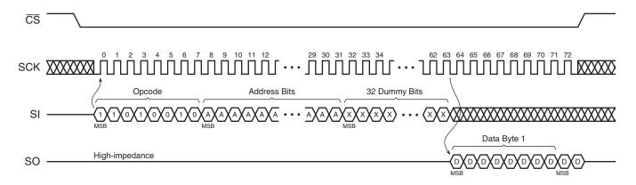
Figure 25-5. Buffer Read (Opcode D4h or D6h)
