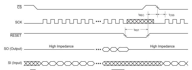
Note: 1. The  $\overline{\text{CS}}$  signal should be in the high state before the  $\overline{\text{RESET}}$  signal is deasserted.
