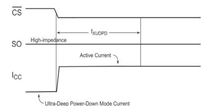
Figure 10-5. Exit Ultra-Deep Power-Down (Chip Select Low)
