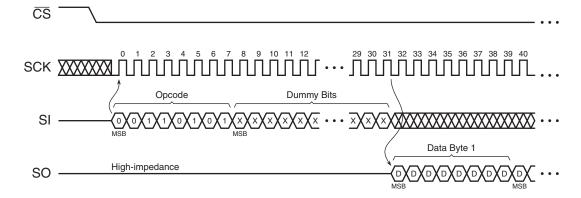
Figure 25-9. Read Security Register (Opcode 77h)
