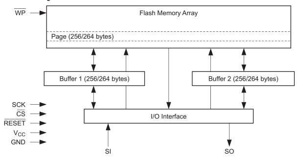
Figure 23-2. Buffer Write
