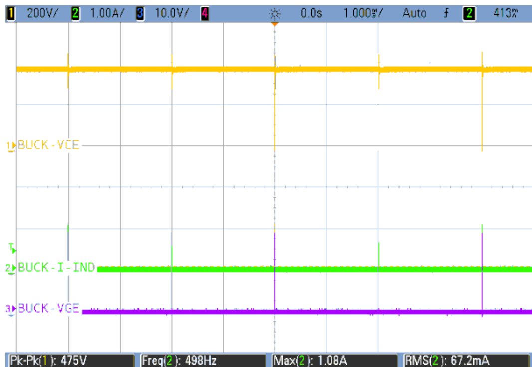
Figure 43. Buck converter - Digital dimming - V_{CE} vs I_{INDUCTOR} vs V_{GE} at 0.5%
