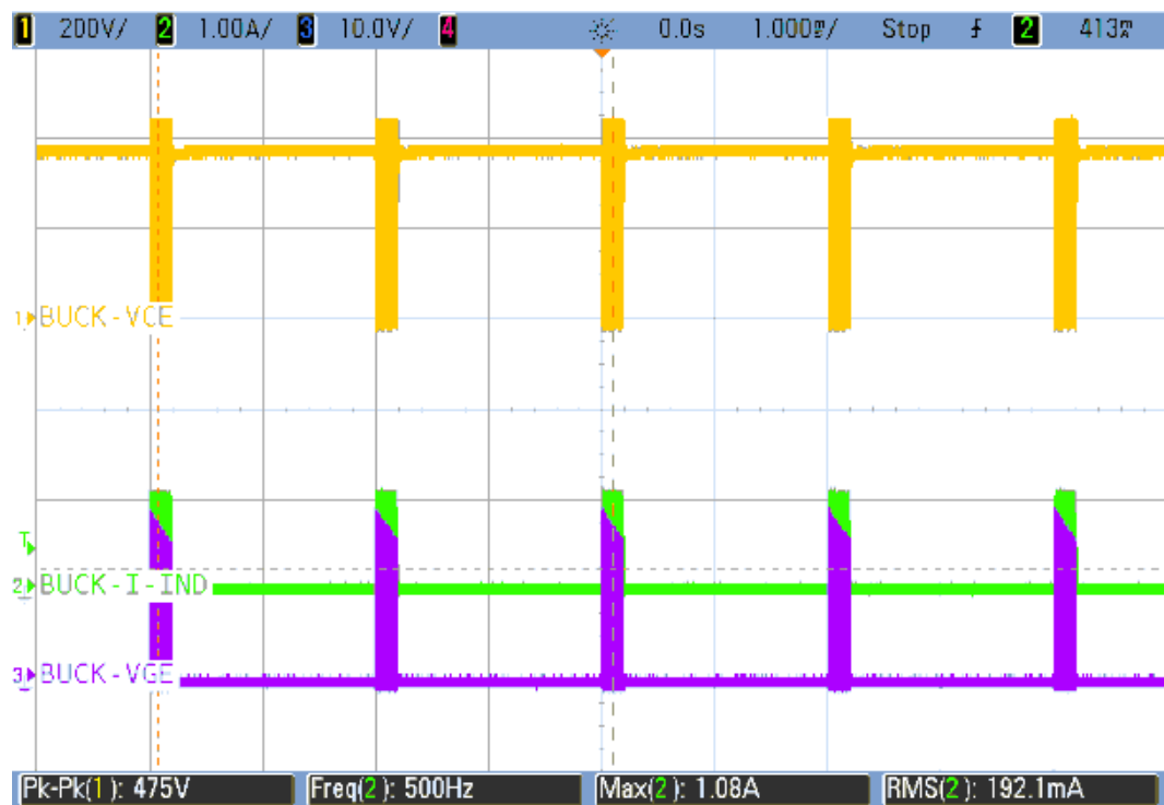
Figure 42. Buck converter - Digital dimming - V_{CE} vs I_{INDUCTOR} vs V_{GE} at 10%
