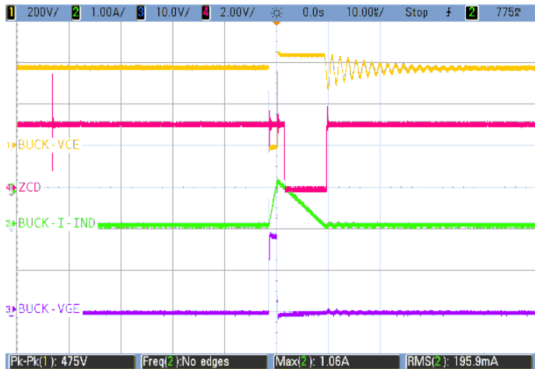
Figure 44. Buck Converter - Digital dimming - V_{CE} vs I_{INDUCTOR} vs V_{GE} vs ZCD at 0.5% - Zoom
