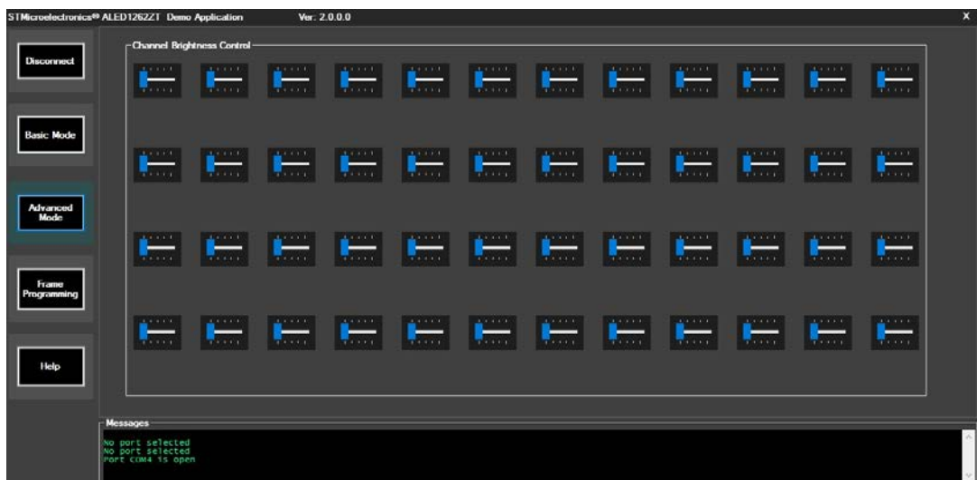
Figure 13. STSW-LLL002GUI advanced mode
