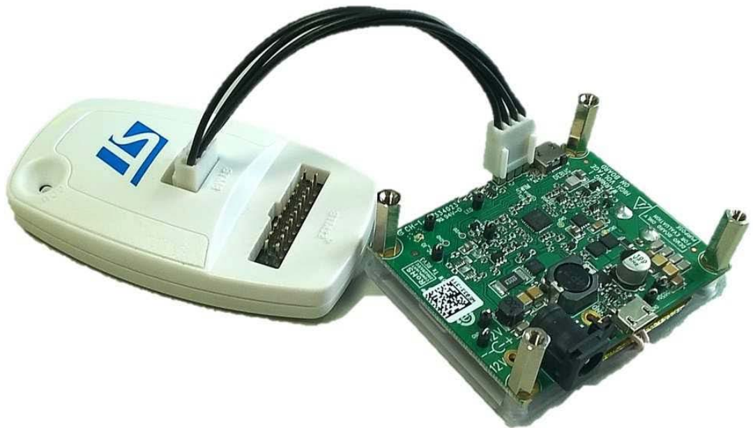
Figure 17. STEVAL-ISB044V1 evaluation board: ST-LINK connection
