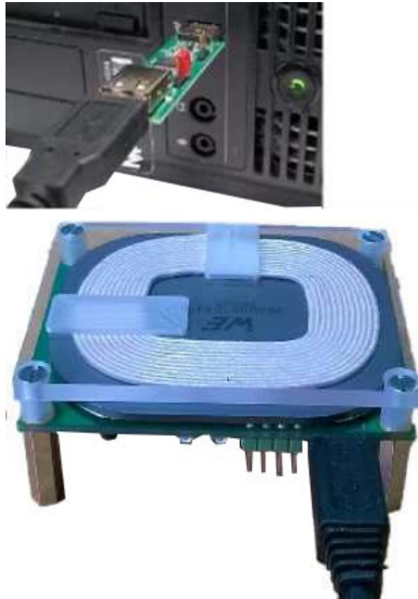
Figure 14. USB-to-UART dongle to STEVAL-ISB044V1 connection
