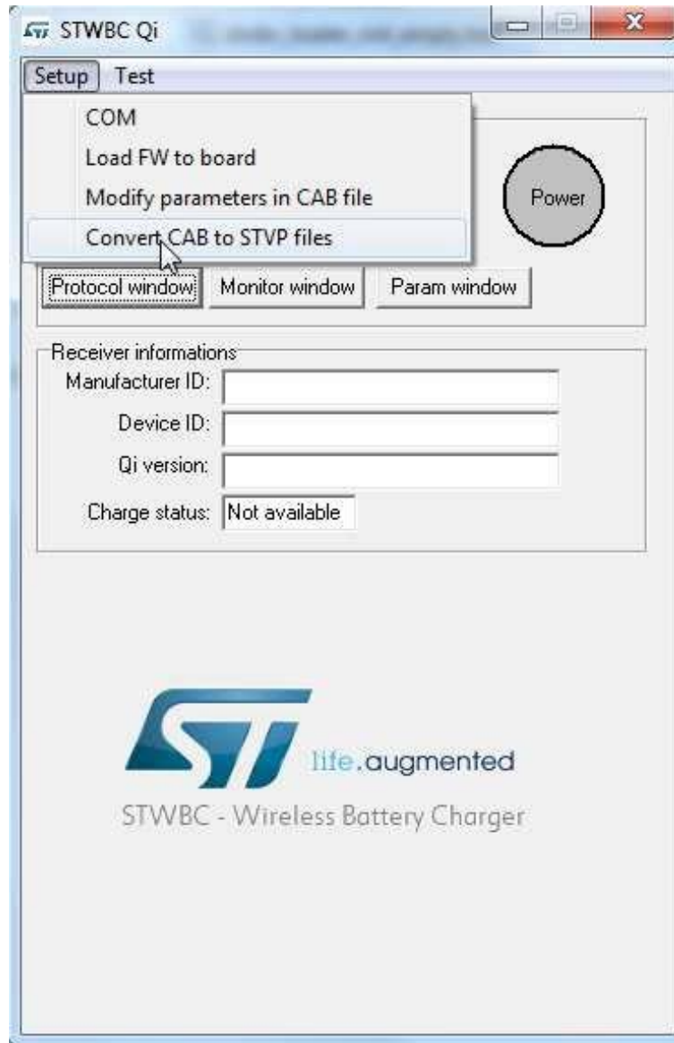
Figure 24. STSW-STWBCGUI: convert CAB to STVP files
