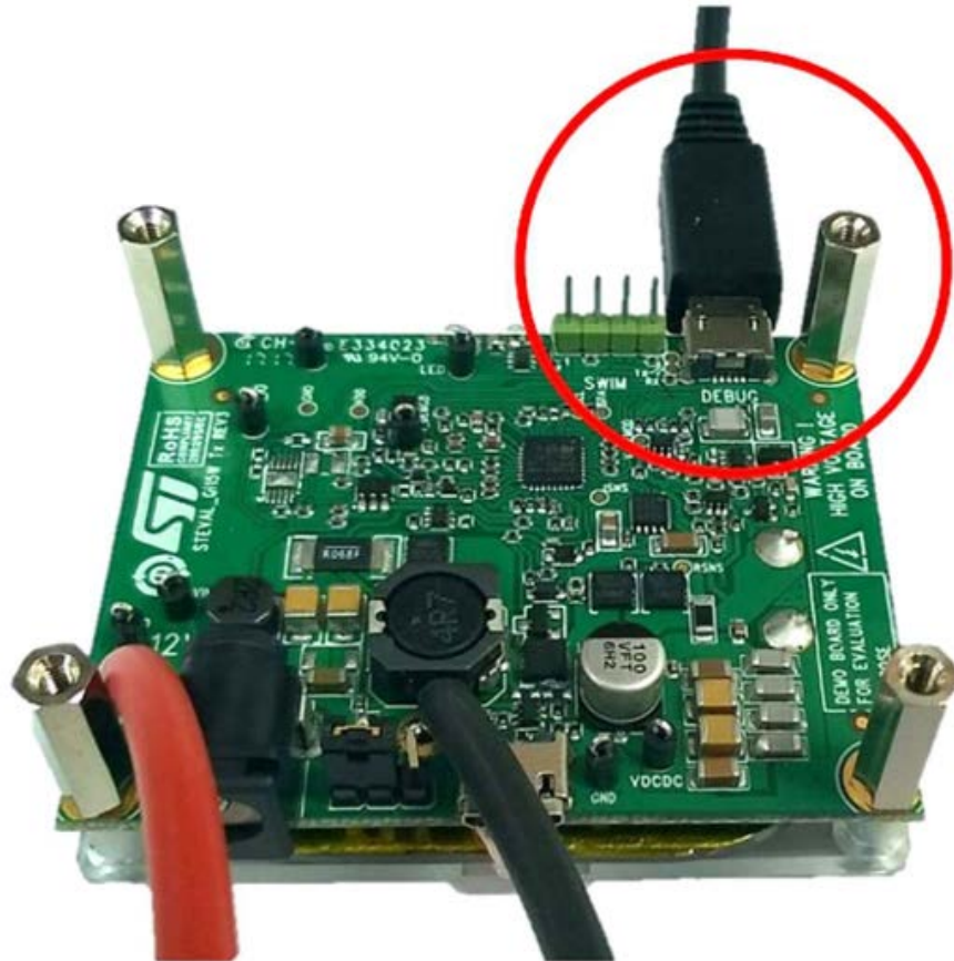
Figure 32. STEVAL-ISB044V1 evaluation board: UART connection
