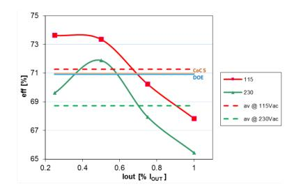
Figure 12. Active mode efficiency vs VIN and comparison with CoC5 and DOE
