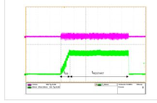
Figure 22. OLP: short-circuit removed and auto-restart
