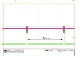
Figure 21. Output overload maintained: t<sub>SS</sub> and t<sub>OVL</sub>
