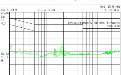
Figure 29. EMI measurements with average detector @ 115 VAC, full load,  $T_{AMB}$  = 25 °C
