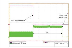
Figure 20. Output overload maintained:OLP steady-state
