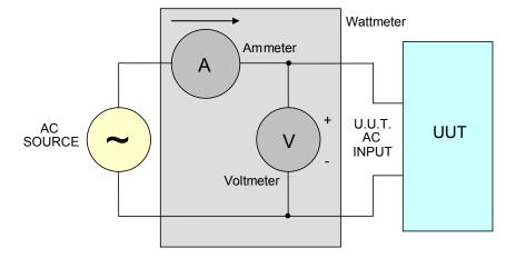
Figure 33. Switch in position 2 - setting for efficiency measurements
