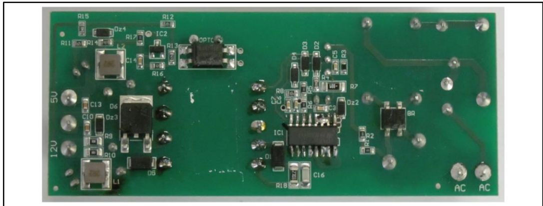
Figure 4: STEVAL-ISA184V1 power supply board (bottom layer)
