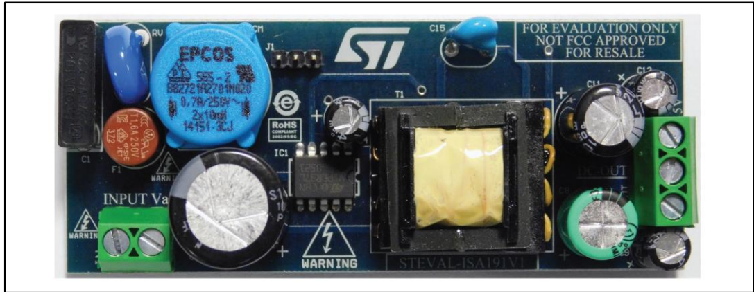
Figure 2: STEVAL-ISA191V1 power supply board (bottom layer)
