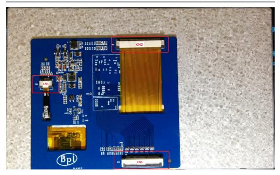
CN2: LCD connectorCN5: TP connectorCN1: Bpi connector
