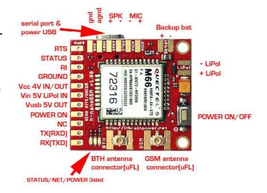
GSM SHIELD (nano) h-nanoGSM v 1.08 top PCB view
