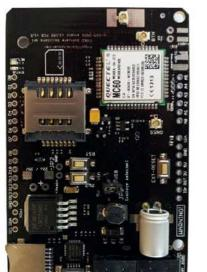
Integrated GSM antenna and uFL connector for external antenna
