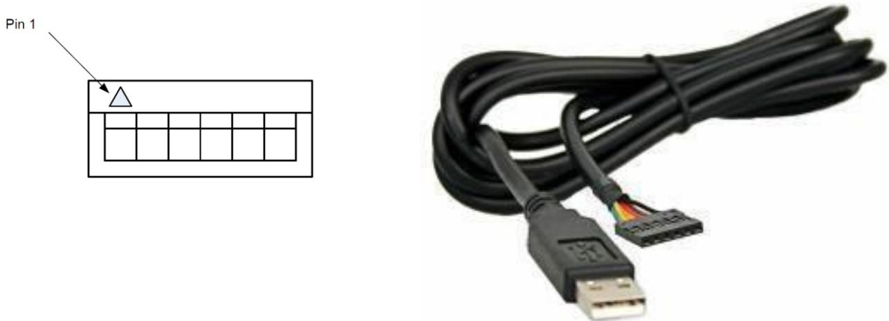
FIGURE 13 - PIN HEADER SOCKET BOTTOM VIEW
