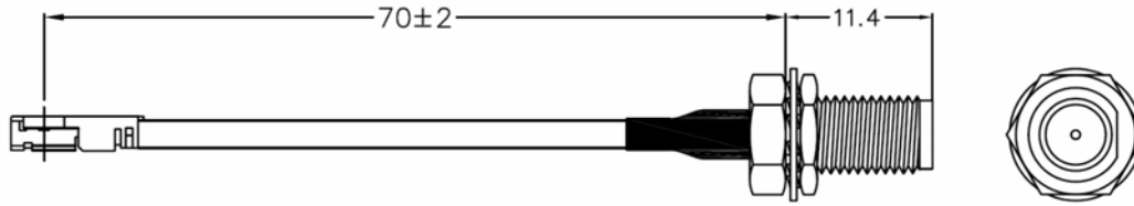
FIGURE 5 – I-PEX MHFIII™ TO SMA-TYPE ADAPTOR MECHANICAL OUTLINE
