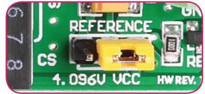
Figure 4-2: Ref. voltage is VCC
