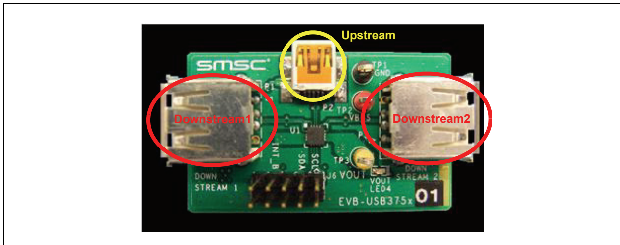
Figure 2.1 Upstream and Downstream Ports
