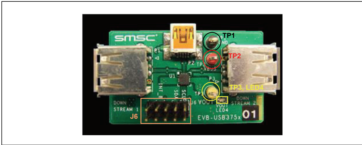
Figure 2.2 Test points, LED and Header
