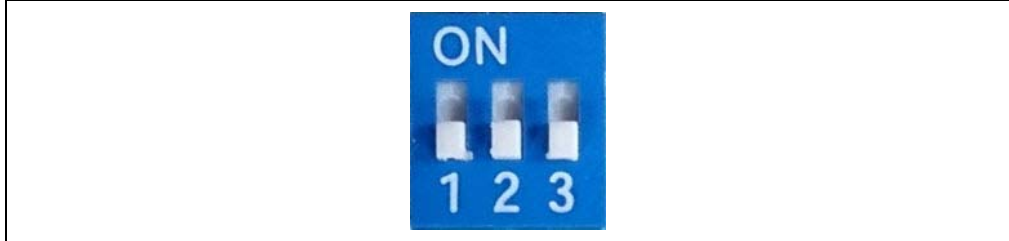
FIGURE 3-1: SW9 IN FLASH APPLICATION MODE
