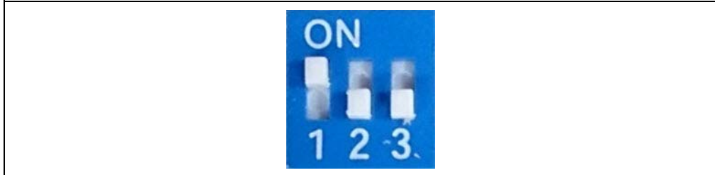
FIGURE 3-29: SWITCH SW9 IN TEST MODE
