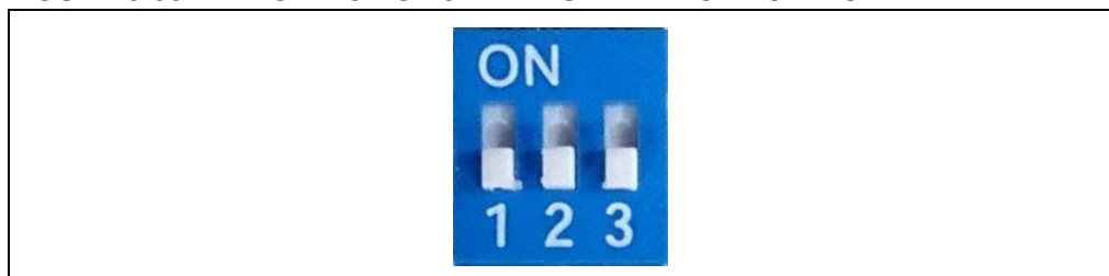
FIGURE 3-35: SWITCH SW9 IN FLASH APPLICATION MODE
