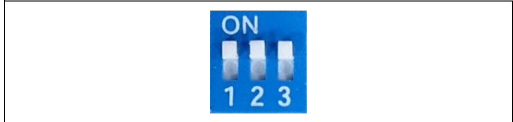
FIGURE 3-36: SWITCH SW9 IN WRITE FLASH MODE
