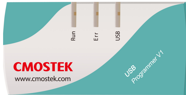
Figure 27. LED Indicators on the USB Programmer
