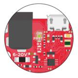
**ON** LED turns on when the FLUO WI-FI is powered up
