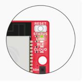
LINK LED remains turned on when your FLUO WI-FI is connected to your wireless network
