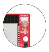
**STATUS** LED turns on when the firmware is running
