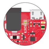
**PRST** LED turns on when both the ATmega644p and the ESP-32 have successfully rebooted.
