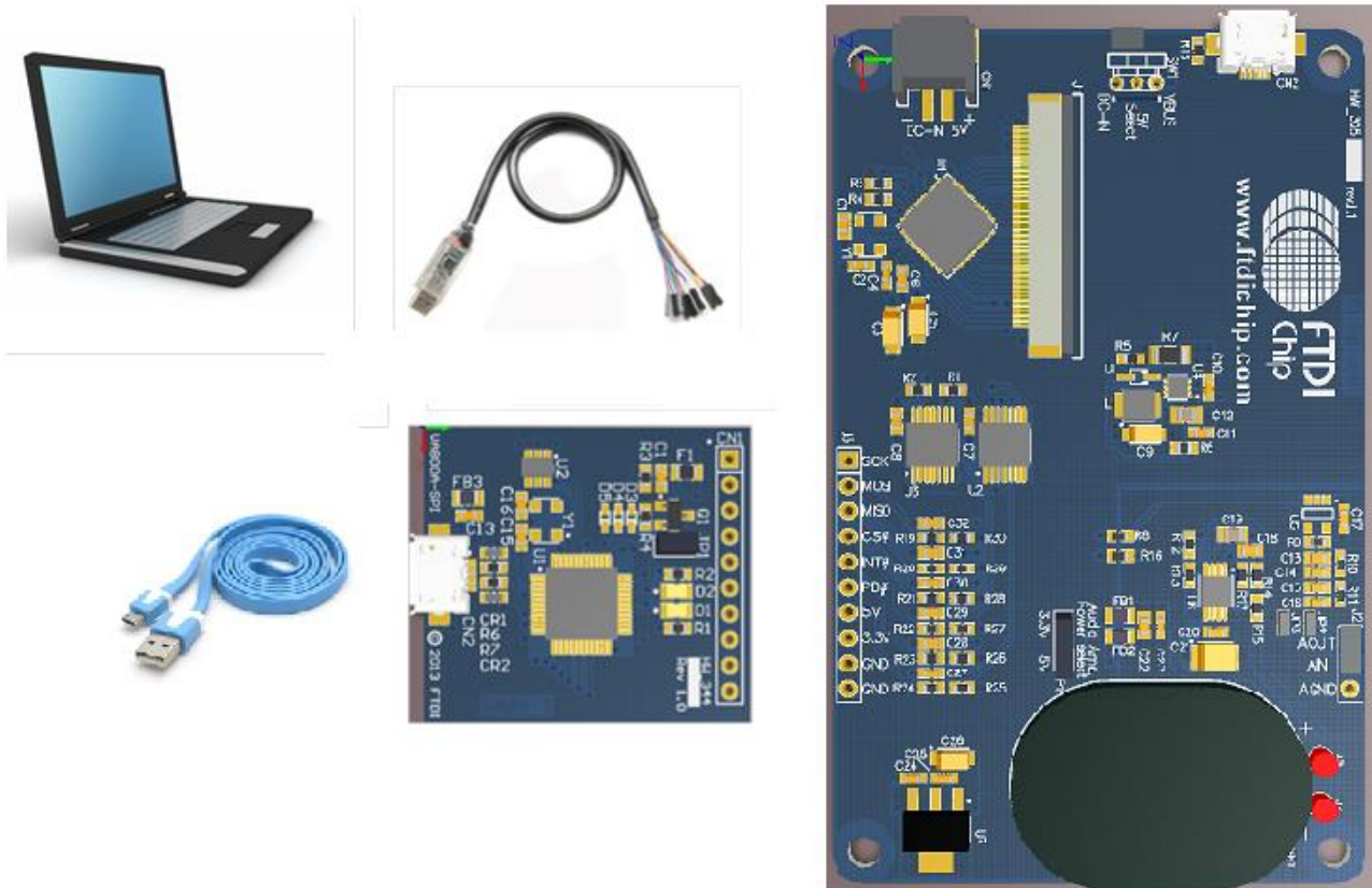
Figure 5-1 – VM810C connects to PC via VA800A-SPI or MPSSE cable.
