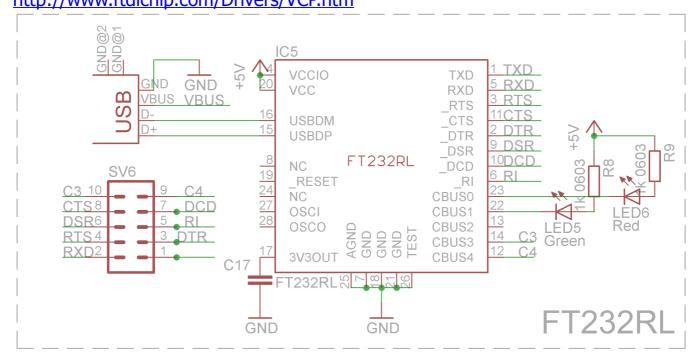
In addition, the system FT232RL lines were derivedXD, TXD, C3, C4, CTS, DSR, RTS, DCD, RI, DTR to the gold pins. These lines are used for emergency programming microprocessor but can also be used for any purpose.
